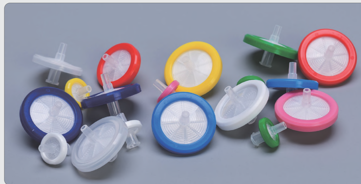
Different color outer rings correspond to different membrane types, and are easy to distinguish and identify
